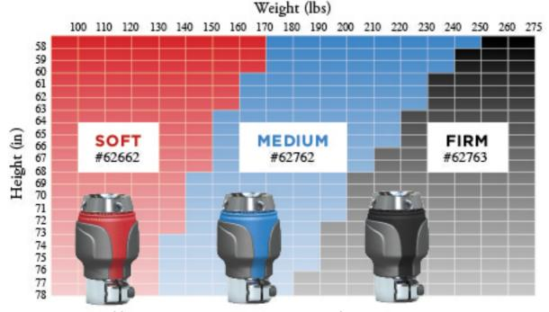
The amount of force applied to the spring pack in the Sfx is based on patient weight and height. This chart shows the spring pack selection based on these patient variables.
